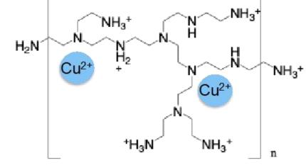
3: Bound Cu(II) ions: increases charge density, anti-fouling
