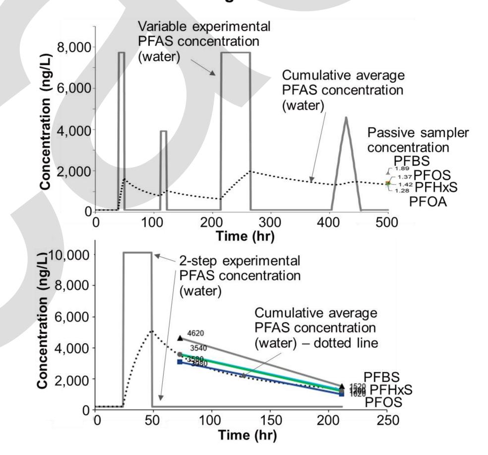
PFAS concentration profile during variable-concentration experiments demonstrate integrative (time-weighted) behavior of passive sampler.
